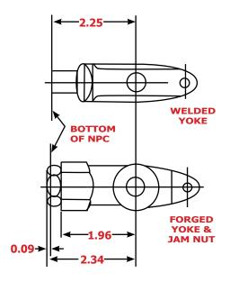
Units manufactured with a "welded" yoke have preset "Y" dimension, measured from the bottom of the NPC to the center-line of the yoke pin, of 2.25 - inches. Because the "Y" dimension is relatively short, the corresponding "X" dimension, measured from the bottom of the NPC to the end of the rod, will also be short, at approximately 34 of an inch.
