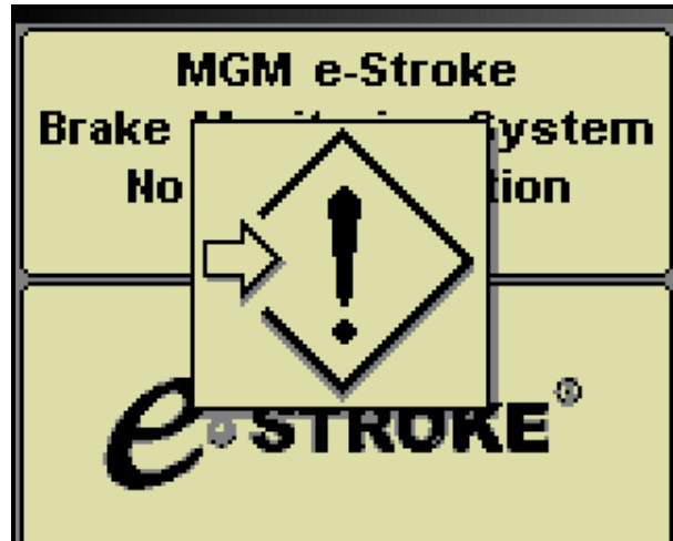
Figure 3: Display Communication Failure Screen
