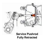
When measuring stroke in this condition, the inspector will observe only the relative difference between the non pressurized and applied positions. This is known as relative stroke. It is important to consider that the travel limit on a brake actuator is based on absolute stroke, not relative stroke.
